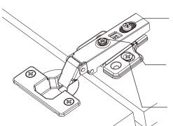
Depth Adjustment Rotate the hinge arm cam to increase or decrease door gap. Horizontal Adjustment
