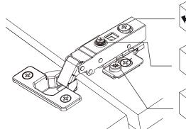
**Depth Adjustment** Move the hinge laterally to adjust door gap.
